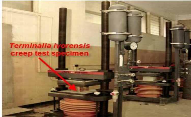
Plate 1.0: Set-up of Creep Testing Machine
