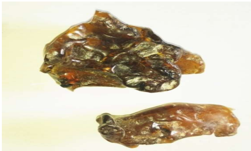
Plate XI: Sample of glass softened by furnace heat
