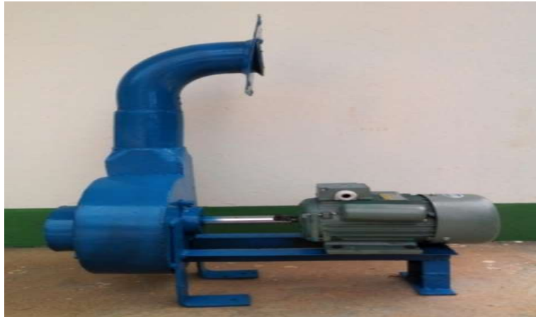
Plate IIX: Complete Centrifugal Fan coupled with electric motor
