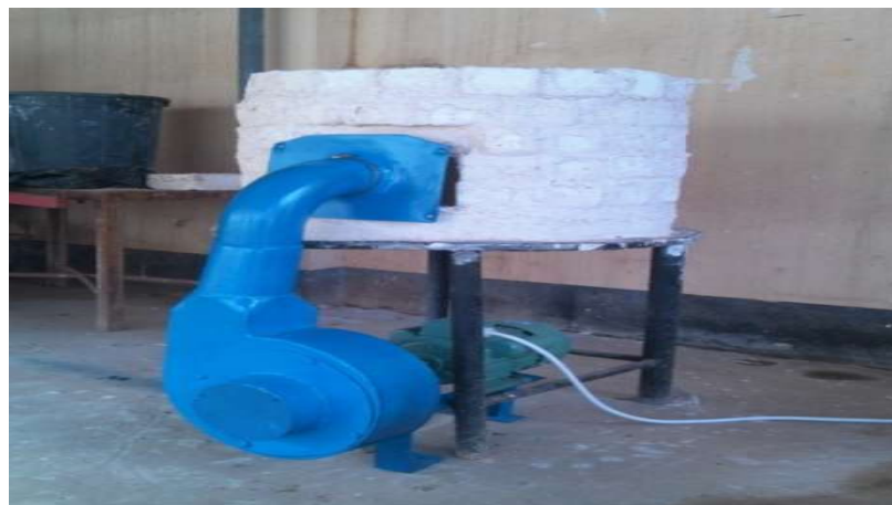
Plate IX: Centrifugal Fan coupled with Modified furnace structure
