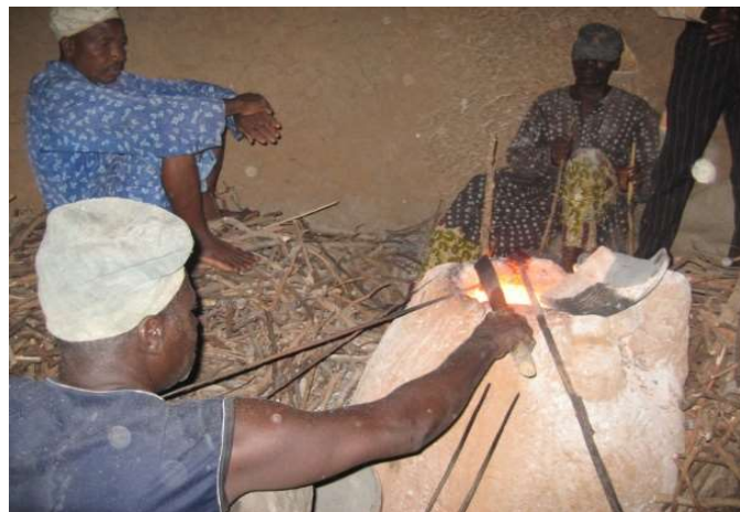
Plate I: Masaga Glass bead making Furnace in operation. Source: Alemaka (2009)
