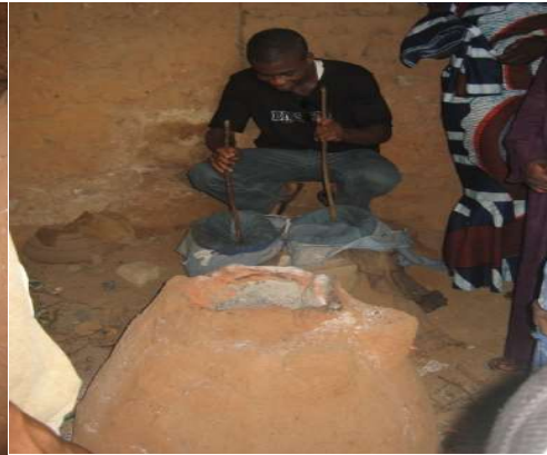
Plate IIb: Manual working of Bellows Source: Alemaka (2009)
