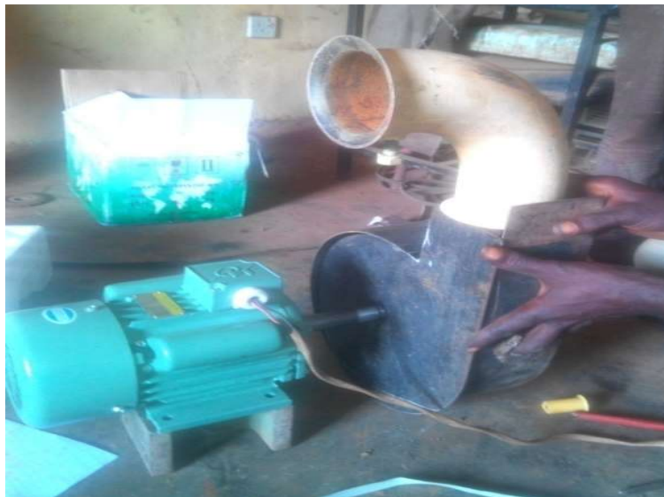
Plate VII: Estimating Elbow welding height
