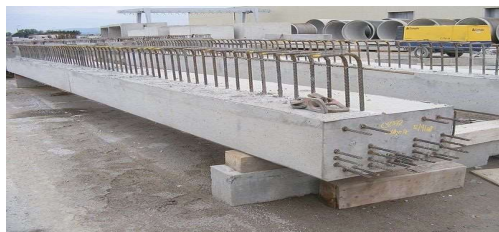
Figure 1- A Typical appearance of a Prestress Beam
