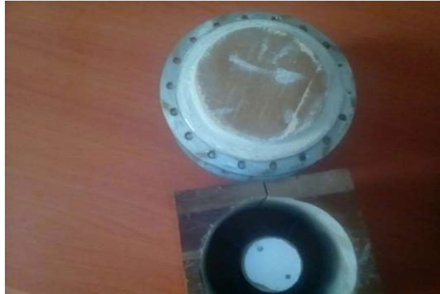
Plate 1: Pattern and the assembled core box.
