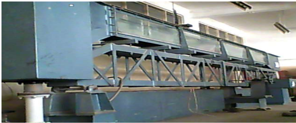
Plate I: Side view of the Tilting Flume
