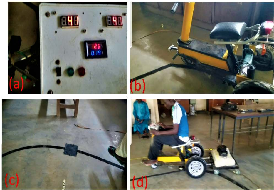
Figure 4: (a) Speed regulated to 41 m/s, (b) Robot on Sharp Corner, (c) Robot on Curved Corner (d) Robot with 150 kg on a sharp corner
