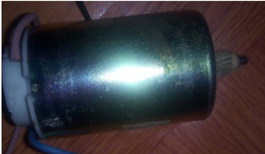
Fig. 6: A 12 V 3 A 2900RPM Permanent Magnet brushed DC motor
