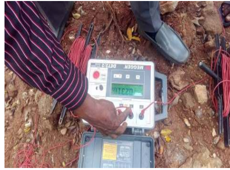
Plate 2: Display of readings of soil resistivity on Megger DET2/2 Auto Earth Tester
