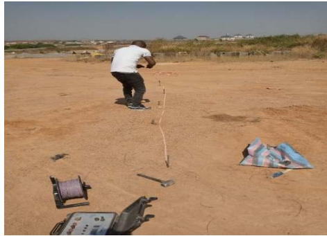
Plate 1: Resistivity measurement at Site
