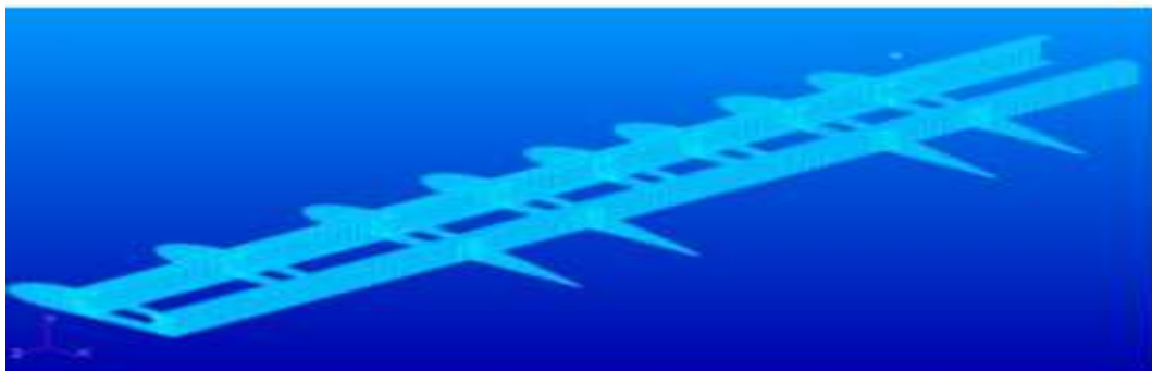
Figure 10: Finite Element of the Wing [7]
