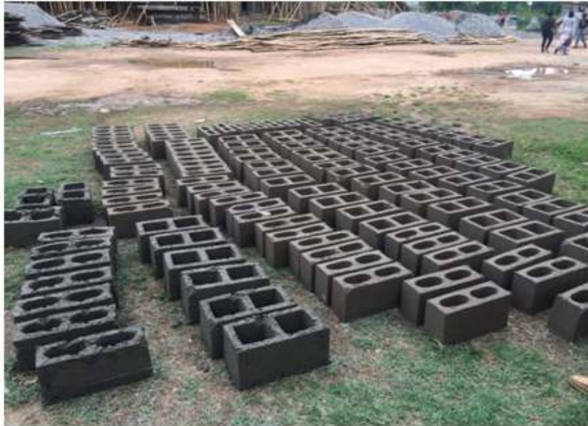
Figure 3: Freshly molded concrete hollow block (CHB) and sandcrete hollow blocks (SHB)
