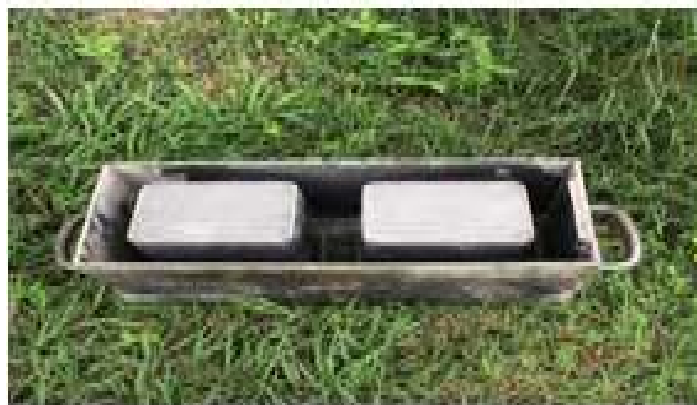
Figure. 1: 9 inches hollow block metal mold
