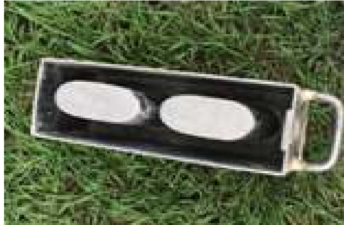
Figure. 2: 6 inches hollow block metal mould
