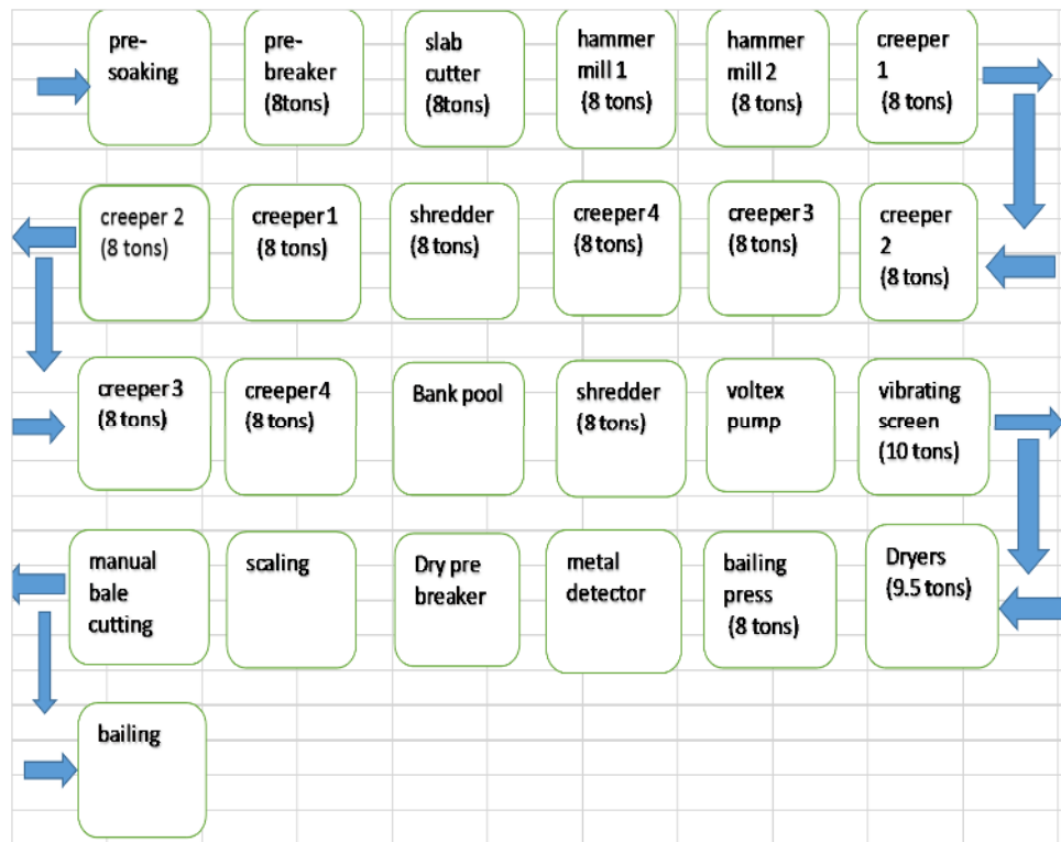
Figure 11: Flow chart for a rubber processing line
