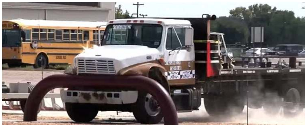
Figure 2.6: A vehicle barrier stopping a truck
