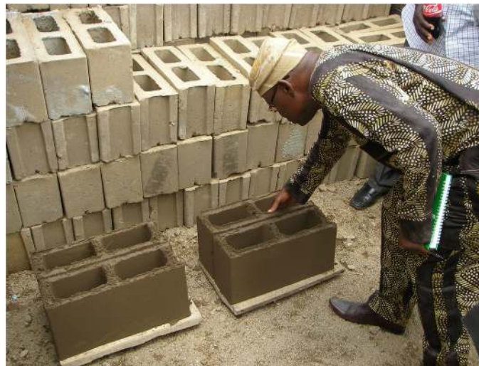
Figure 2.1: Typical sandcrete units in Nigeria (Crist, 2013)
