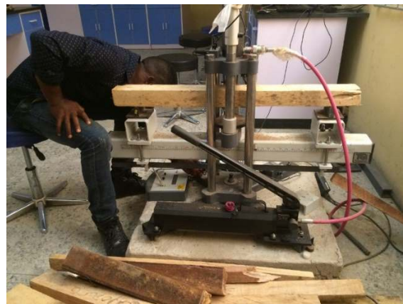
Figure 6: Datum check for the flexural testing machine
