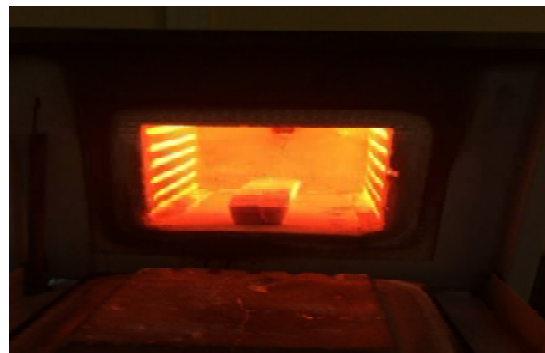
Figure 3: ELF furnace showing the final stage of charr
