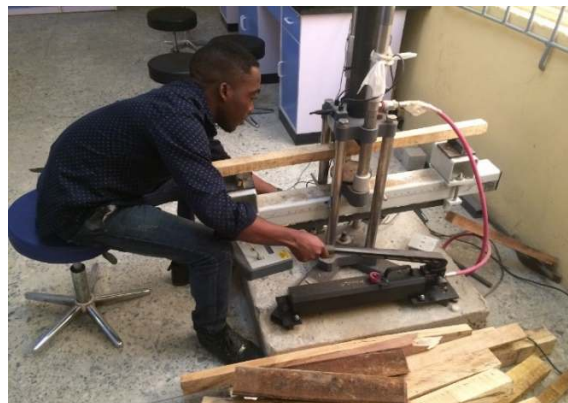
Figure 5 : Application of load on the wood sample machine and ASTM 293 C
