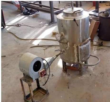
Plate 4a & 4b: The produced crucible furnace before and after painting
