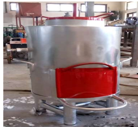
Plate 4a & 4b: The produced crucible furnace before and after painting
