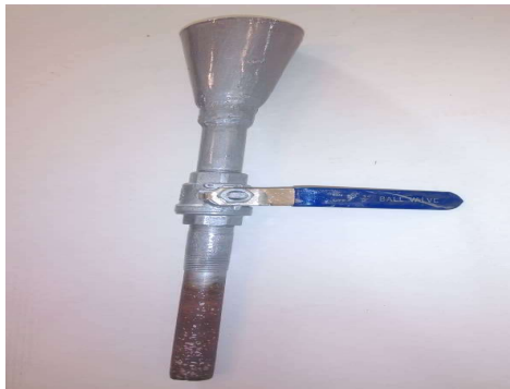
Plate 3c: Coupling from blower to burner.
