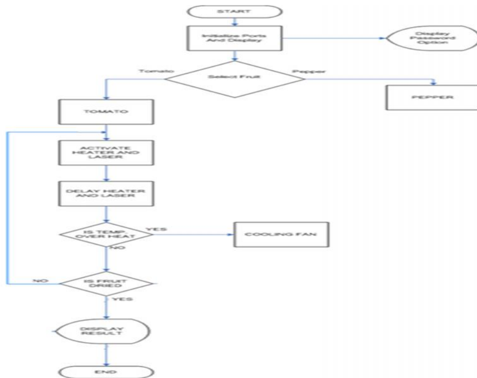
Fig. 5 Flow chart for programming the microcontroller
