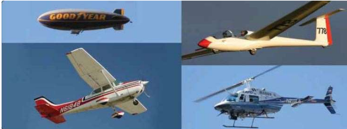
Figure 2: Examples of different categories of aircraft, clockwise from top left: lighter-than-air, glider, rotor-craft, and airplane.
