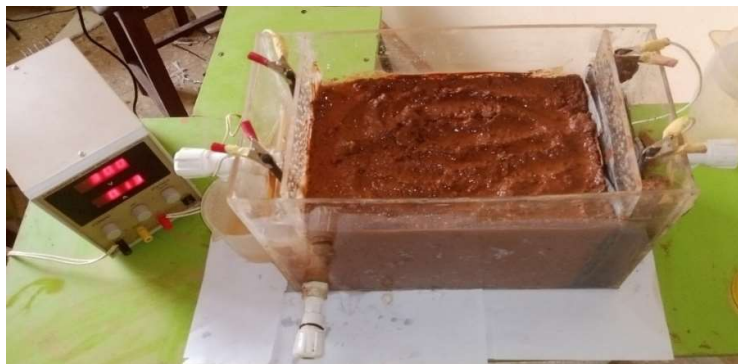
Figure 1: Chelant Enhanced EK Remediation of Crude-oil Contaminated Soil
