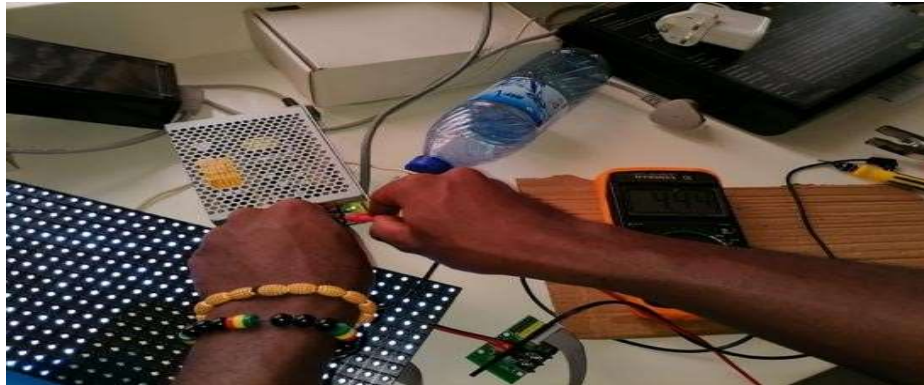
Figure 9: Picture of Testing the Voltage of the Power Supply with a Multimeter
