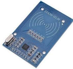
Figure 3: RFID card Reader
