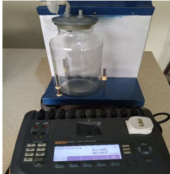
Figure 4: Electrical safety test arrangement
