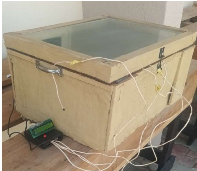
Plate 4.2: IoT monitoring interface on solar box cooker experiment
