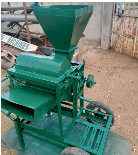
Figure 2: pictorial view of the manually operated mobile maize shelling machine Evaluation of the machine
