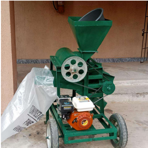
Figure 1: pictorial view of the motorized mobile maize shelling machine
