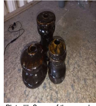
Plate III: Some of the sample insulators produced
