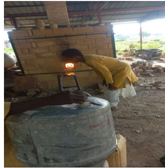
Plate II: Kerosine firing being regulated
