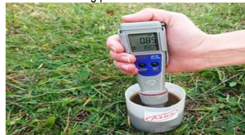
Plate 1: Measuring pH value using pH meter
