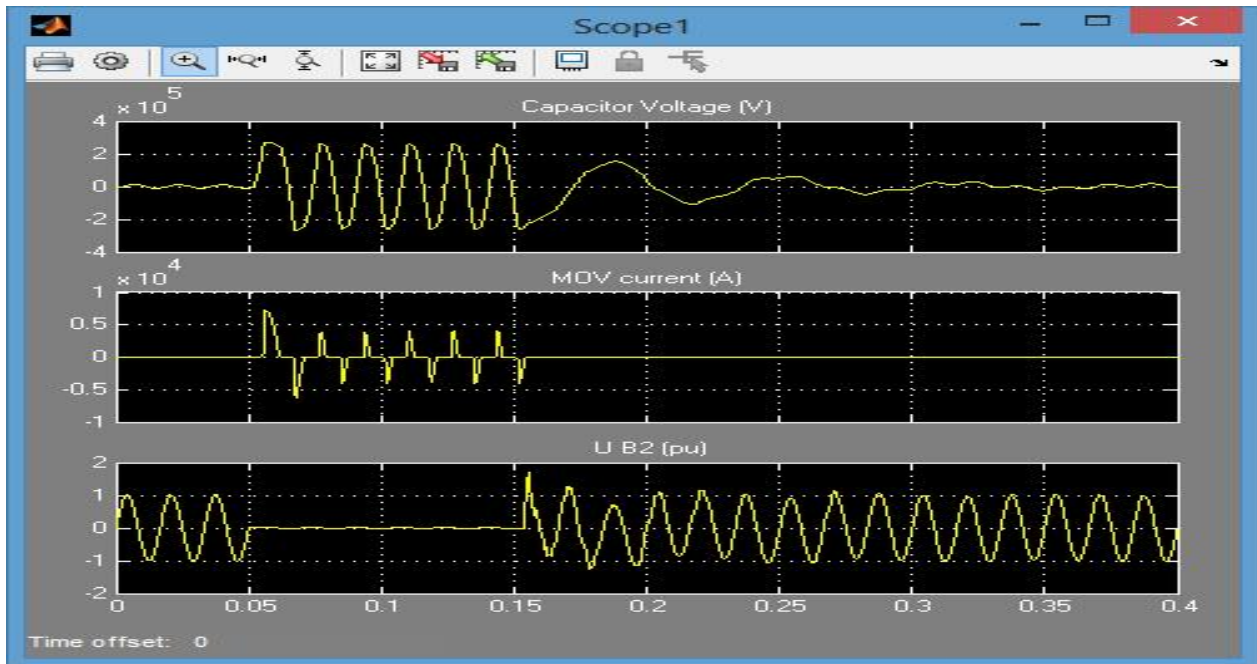
Figure 5: MOV conducting at half cycle producing voltage across the capacitor in Scope 1
