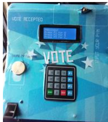
Figure 6: Finished standalone biometric e-voting
