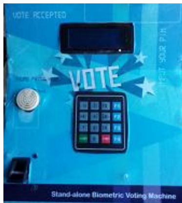
Figure 6: Finished standalone biometric e-voting
