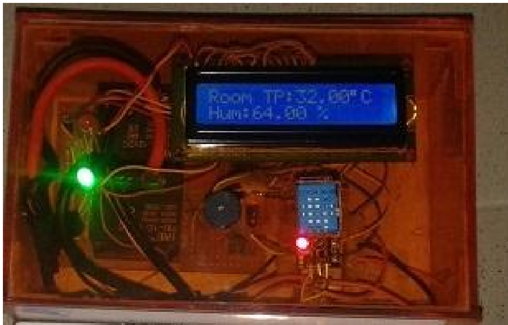
Figure 4: Assembled Thermal Comfort System
