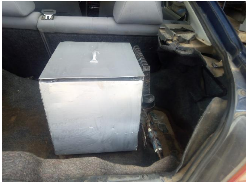
Plate: 1: The vapor absorption refrigerator fitted to the car
