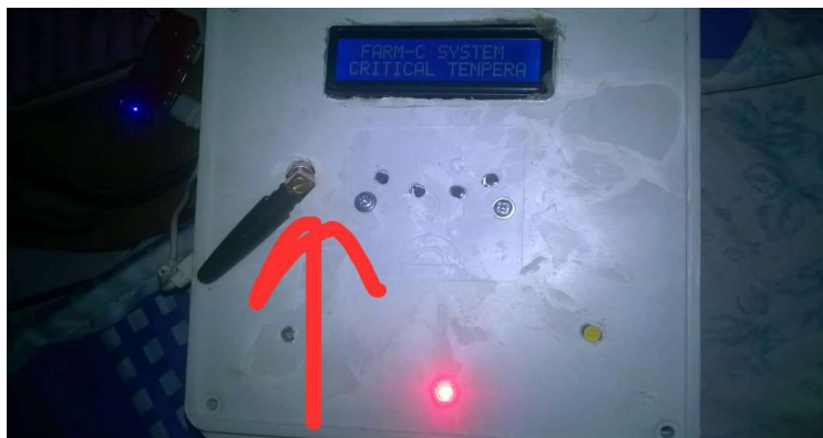
Figure 4.4: The prototype of the Soil Moisture Detector System using Temperature and PH sensors, with SMS alert Notification System.
