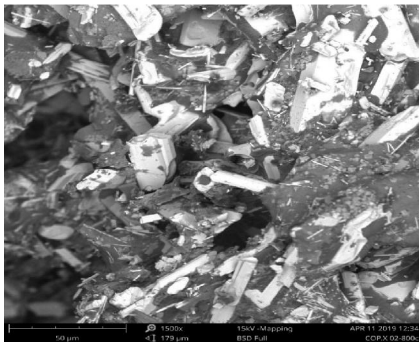
Figure 6: SEM image of \text{Bi}_{0.6}\text{K}_{0.2}\text{Ba}_{0.2}\text{FeO}_3 nanoparticles annealed at 800 °C
