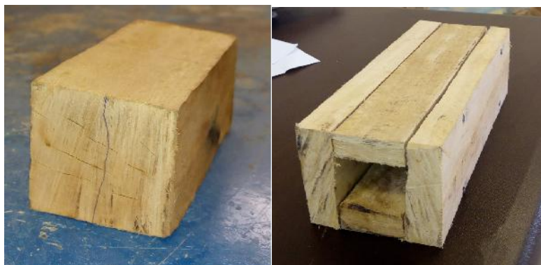
Plate 1: Showing Solid-Section Test Specimen Plate 2 Showing Box Section Test Specimen
