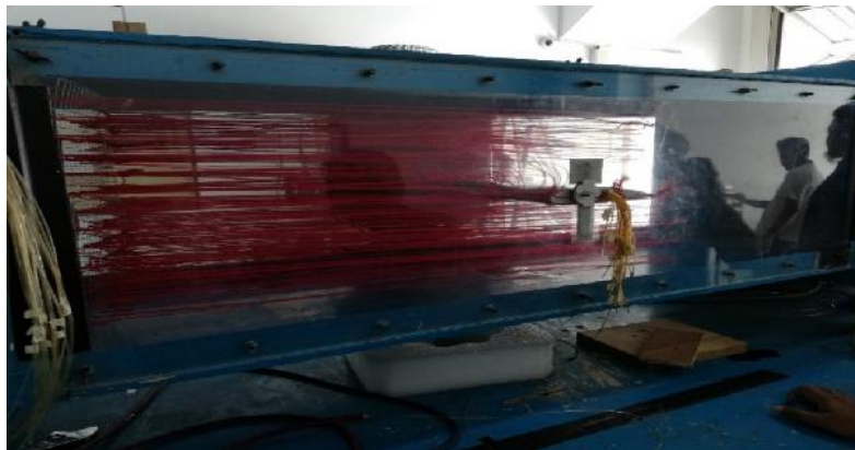
Figure 4: Tuft set up in the wind tunnel
