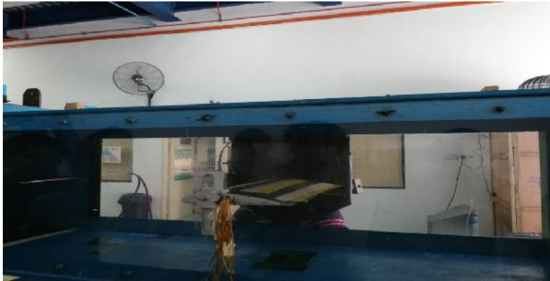
Figure 3: Installed wing model in the open return wind tunnel
