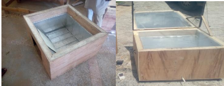
Fig. 4: Box unit with PCM tank before and after glazing
