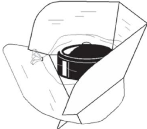
Fig.1. Panel Solar Cooker (SCP, 2015)
