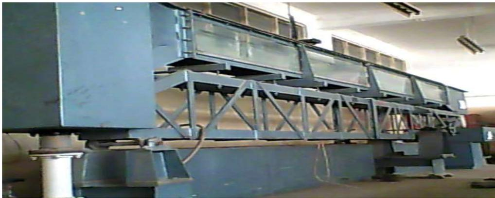
**Plate I:** Side view of the Tilting Flume
