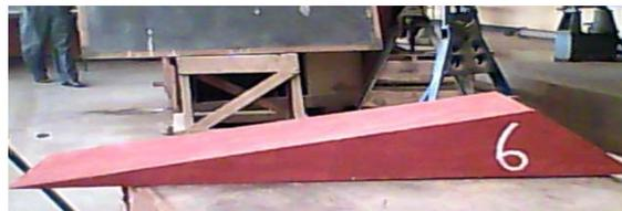
**Plate VII:** Model 6 of apex angle  $130^\circ$ , upstream angle and slope,  $10^\circ$  and 6:1, downstream angle and slope,  $40^\circ$  and 1:1 respectively.
