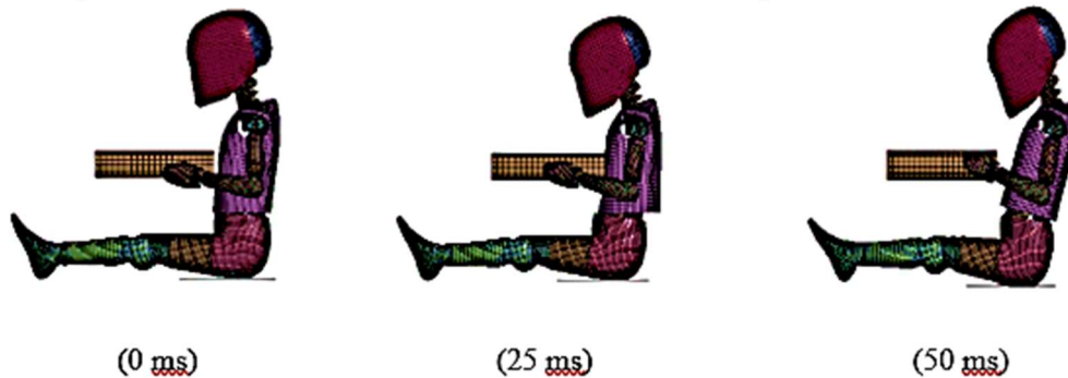
Figure 4: Response of Dummy at Some Instances in the Impact Test
