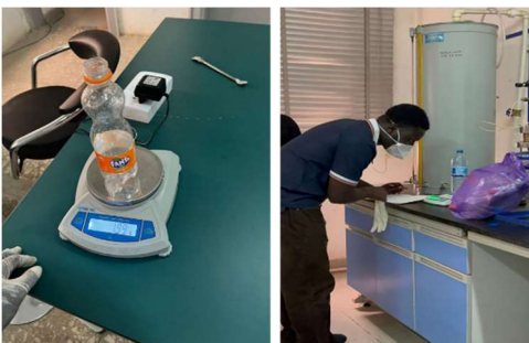
Fig. 3: Measurement of the weights of the plastic wastes
