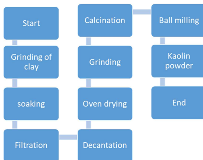
Figure 1: The block diagram for beneficiation/ Preparation of Kaolin Powder.
