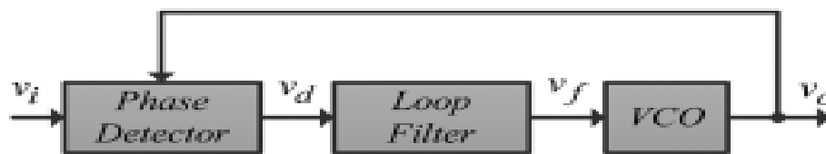
Figure 1: Basic Structure of a Conventional PLL [10].
