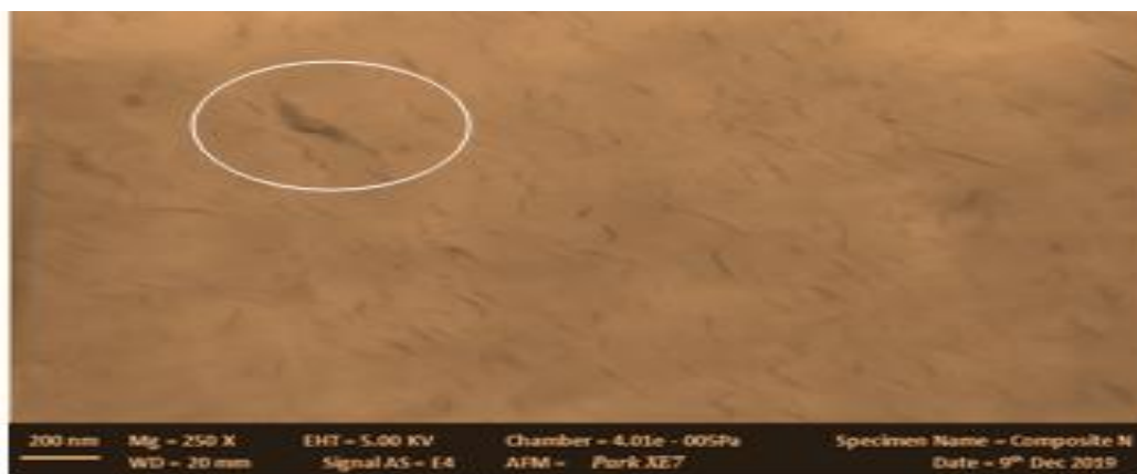
Plate III: SEM Image of Epoxy/nanoclay Composite F (5 wt % epoxy & 95 wt % nanoclay)
