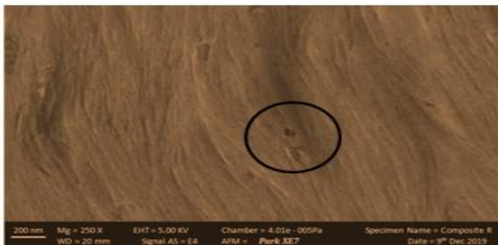
Plate II: SEM Image of S-glass/epoxy Composite F (5 wt % nanoclay & 95 wt % epoxy)
