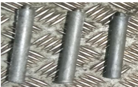
Figure 5: Al-Mg alloy produced from recycled Al and magnesium ribbon
