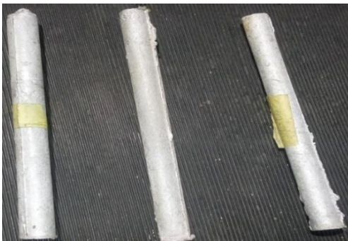
Figure 4: As-cast aluminium ingots
