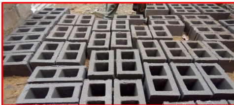
Figure 2: Metakaolin Sandcrete blocks produced at various replacement levels
