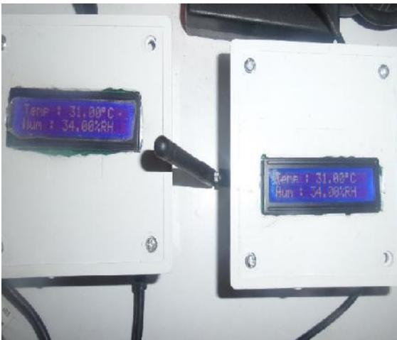
Figure 10b. ZigBee (Tx and Rx) module system packaging
