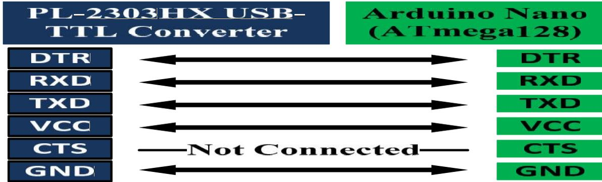
Figure 1: A:Pin configuration of USB-TTL Converter
