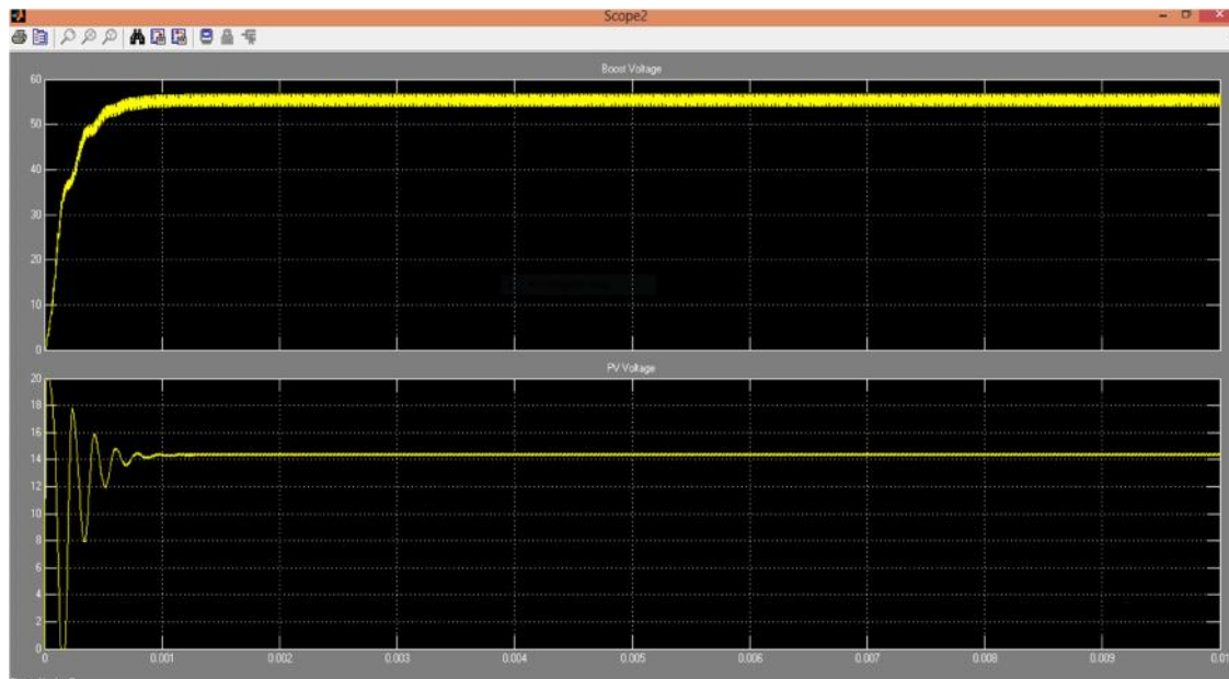
Figure 5: Output Voltages from Boost Converter Using P&O MPPT under Constant Solar Irradiance, 1000W/M 2 and Temperature 25°C
