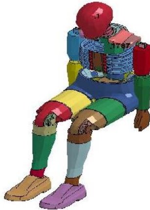
Figure 3: Head and chest accelerometer nodes of HIII dummy FE model (LSTC 2017)
