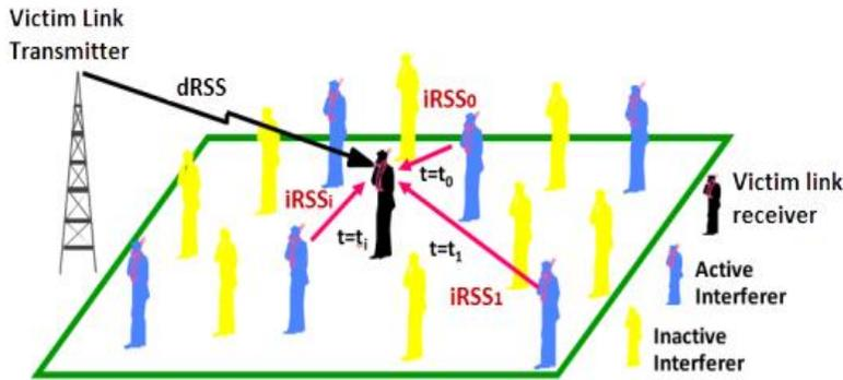
Fig. 1: Typical victim and interferer scenario for a Monte Carlo Simulation trial.
