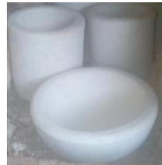
Figure 5: Fired refractory crucibles
