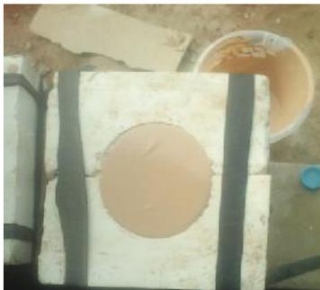
Figure 3: Slip casting of raw materials for crucible
