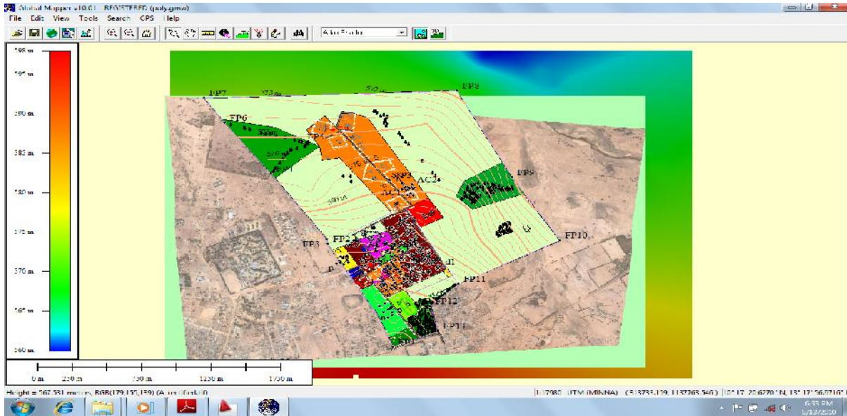
Figure 4a: Satellite image, land use map and topographical map all overlaid on the DTM.
