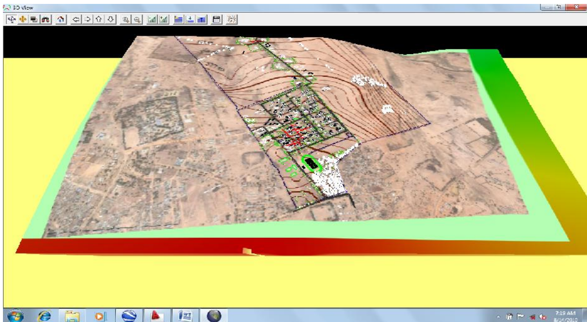
Figure 4b: Satellite image and topographical map all overlaid on the DTM in 3D
